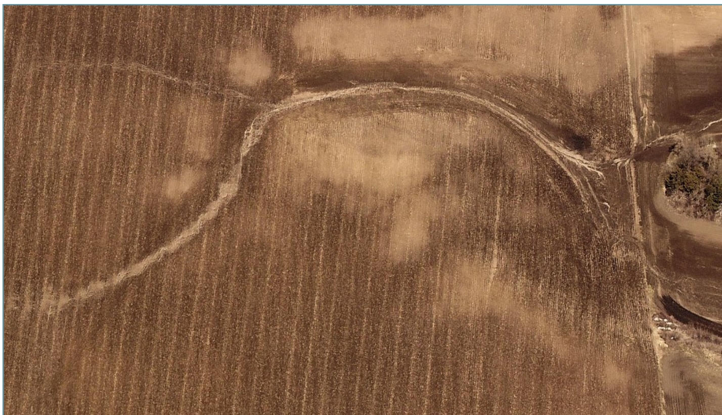
Aerial photo from before the project installation shows the gully through the field. Two basins and a critical area planting were designed to reduce erosion in the field and reduce sediment transport downstream.
