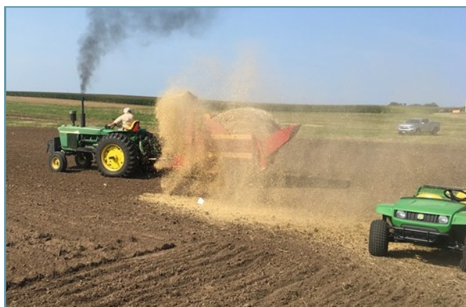
Straw mulch was spread and crimped into the soil to reduce erosion until perennial vegetation is established.
