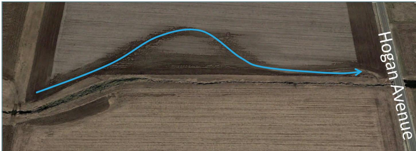
View prior to installation of the project. Sediment build-up along the waterway prevented field runoff from accessing the waterway causing erosion in the field.
